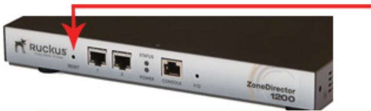
To pin reset your ZoneDirector to factory default configuration, using a straightened paperclip, press and hold the **RESET** button for 8 - 10 seconds then release.
