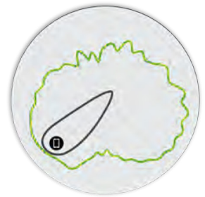
Figure 5. A350 5GHz Elevation Antenna Patterns
